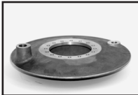
35PA17 Rear Brake Backplate for 270mm Brakes
