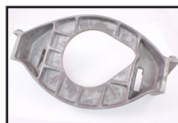
57CH432(CAST) Front Cross Member Oval behind Radiator - CASTING
